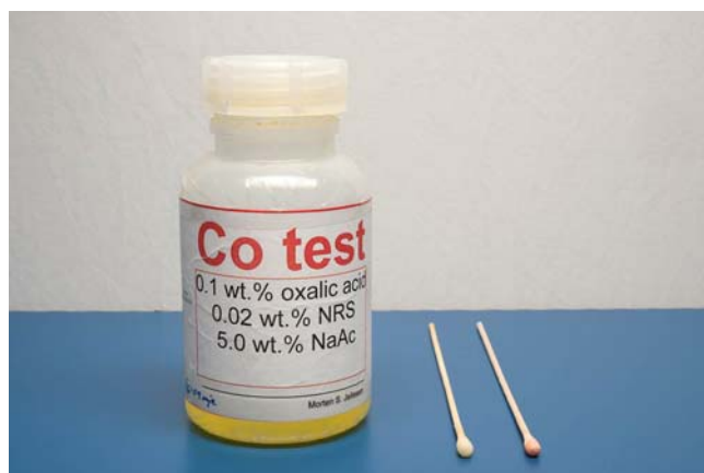
Figure 1. Cobalt spot-test mixture as developed by Dr Jacob Thyssen (photograph provided by Jacob P. Thyssen).
