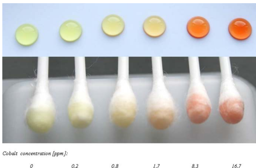
Figure 2. Color is more intense with increasing cobalt level (photograph provided by Jacob P. Thyssen).
